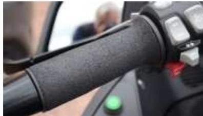
Check the hand grips are intact, securely attached and don't rotate due to the glue deteriorating.
