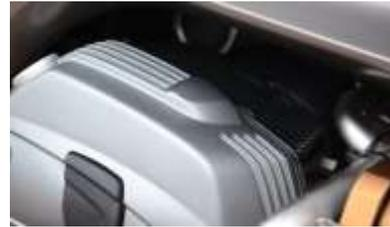
If your bike is air cooled, check the fins and oil cooler radiator matrix are not clogged with debris.
