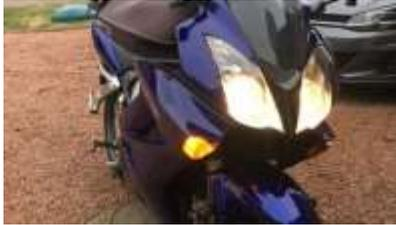
Check daylight running and headlamps, including full beam, are working. Check the horn.
