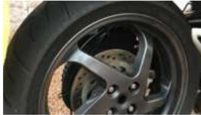
Check front and rear tyres' tread for wear, cuts, nails, squaring off, and side walls for the whole 360° circumference. Check pressures.
