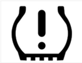
There are two systems in common use, direct sensing and indirect sensing. The direct type uses sensors in each wheel to relay the individual pressures to the system whereas the indirect type uses the ABS sensors to detect long term differences in the rotation of the wheels as a tyre with low pressure has a slightly lower rolling circumference than one at the specified pressure. Both
