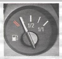
the last drops? The first thing to realise is that fuel gauges are not precise instru-ments. Even in the most modern and snazzy cars, the technology is relatively basic: the level in the
