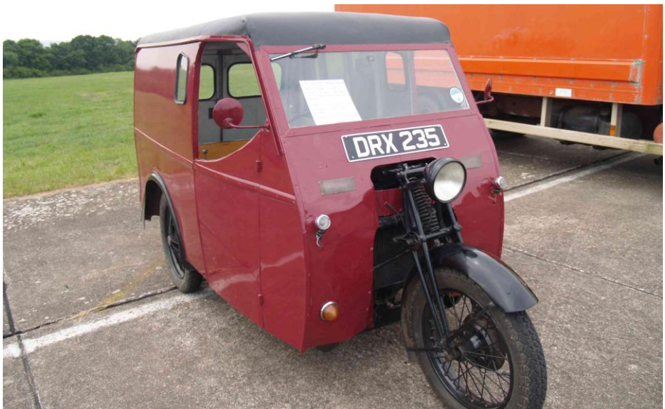
A 1947 Reliant Girder Fork Van equipped with a 748cc 4-cyl side valve engine and crash gearbox
