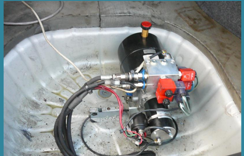
The skid mechanism mounted inside the boot of the skid car
